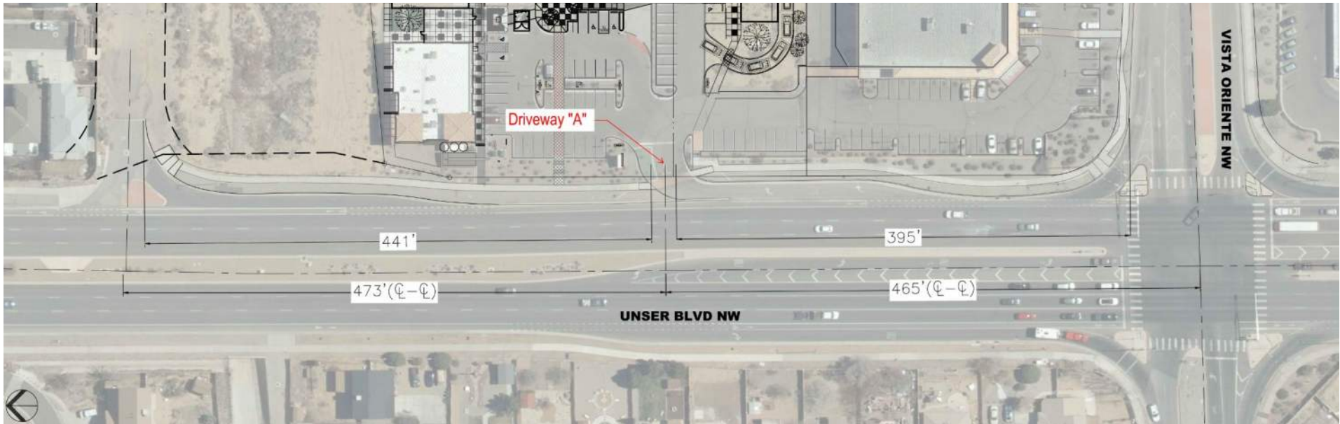
Figure 23 - Access Spacing: Driveway "A"
