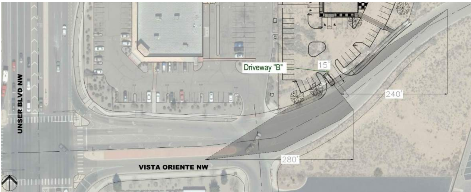
Figure 27 - Sight Distance: Driveway "B"
