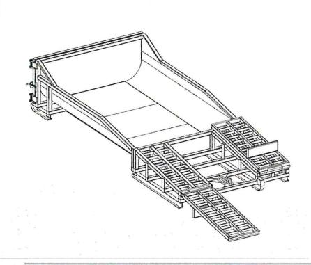
A portable, self-contained and watertight container affixed with ramps that controls, captures and contains caustic concrete wastewater and washout material.
