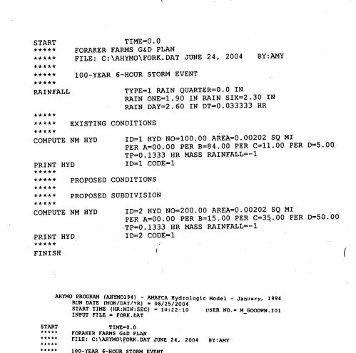
\*\*\*\*\* EXISTING CONDITIONS ID=1 HYD NO=100.00 AREA=0.00202 SQ MI PER A=00.00 PER B=84.00 PER C=11.00 PER D=5.00 TP=0.1333 HR MASS RAINFALL=-1 K = .127917HR TP = .133300HR K/TP RATIO = .959620 SHAPE CONSTANT, N = 3.682038 UNIT PEAK = 4.7994 CFS UNIT VOLUME = .9975 B = 333.38 P60 = 1.9000 AREA = .001919 SQ MI 'IA = .48263 INCHES INF = 1.20137 INCHES PER HOUR RUNOFF COMPUTED BY INITIAL ABSTRACTION/INFILTRATION NUMBER METHOD - DT = .033333 PARTIAL HYDROGRAPH 100.00
