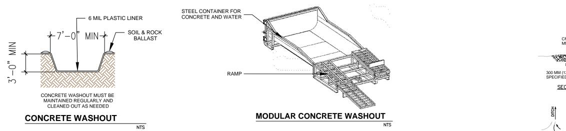
LOCATE WASHOUT AT LEAST 50 FT FROM STORMDRAINS, OPEN DITCHES, WATER BODIES OR PROJECT PERIMETER. A SIGN SHOULD BE INSTALLED ADJACENTLY TO THE WASHOUT.
