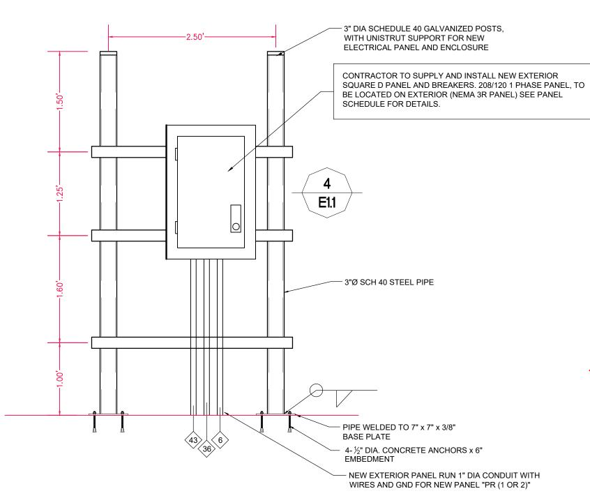
NEW PANEL PR-1 ELEVATION DETAIL
