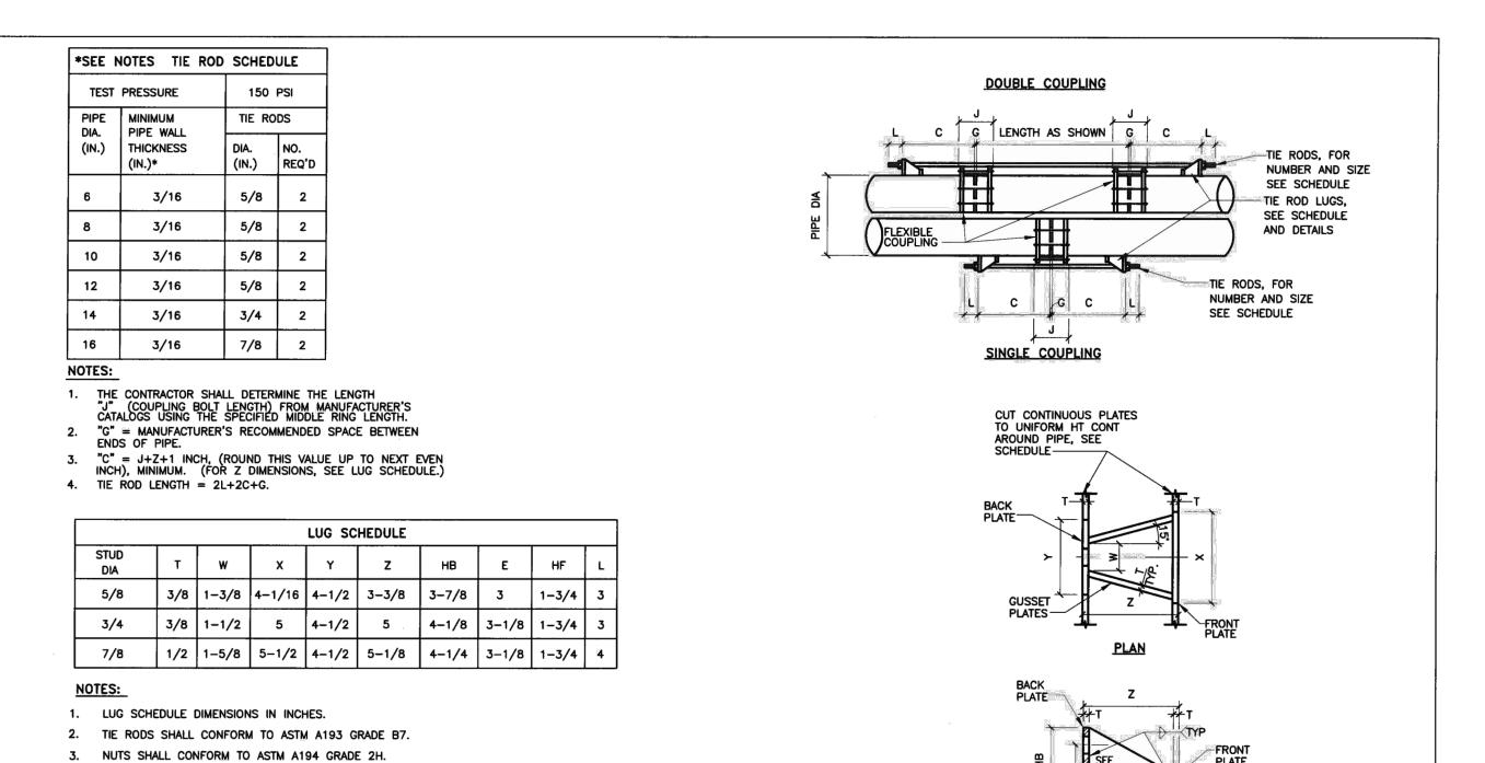
GUSSET PLATES BEVEL AND CURVE BOTTOM TO FIT PIPE
