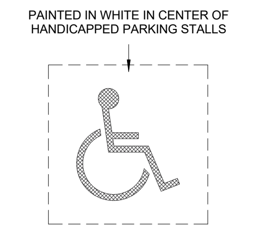
4 Accessible Parking Space Marking 1/4" = 1'-0"
