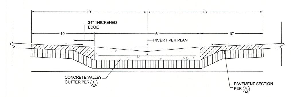
PAVEMENT SECTION - BID ALTERNATE NO. 2
