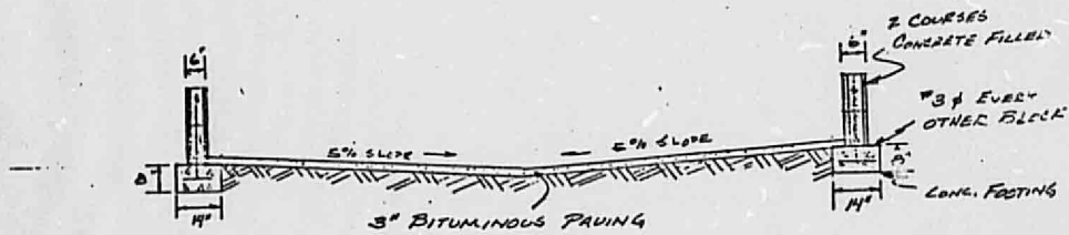
CROSS SECTION 20' DRAINAGE EASEMENTS SCALE 1" = 4'
