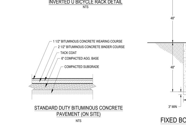
**STANDARD DUTY BITUMINOUS CONCRETE PAVEMENT (ON SITE)**
