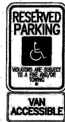
TYPICAL HANDICAP PARKING SIGN (VAN ACCESSIBLE) SCALE: 1" = 0'-6"
