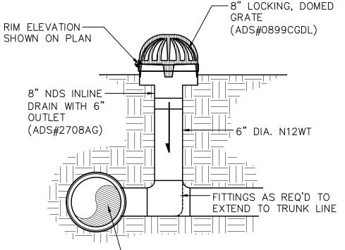
ADS N12WT FITTINGS AS-REQ'D TO CONNECT TO ADS N-12 STORM DRAIN MAIN. SEE DETAIL FOR PIPE DIAMETER.
