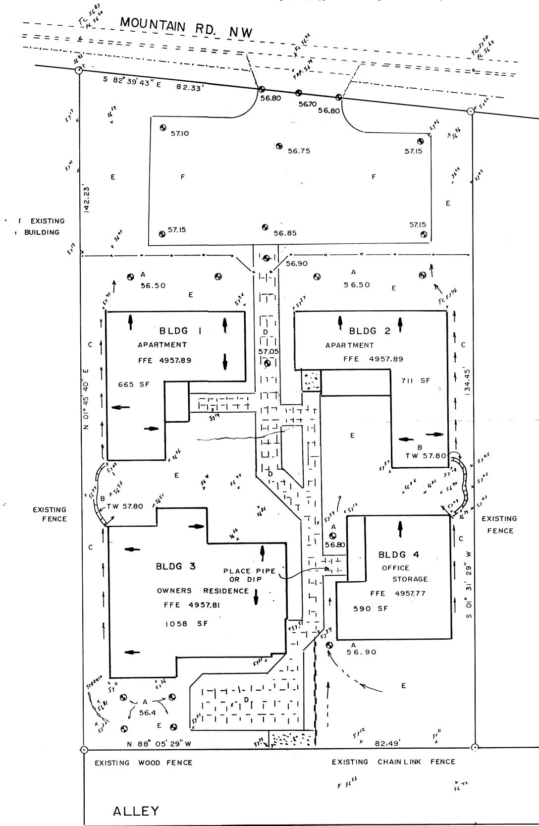
The purpose of this grading and drainage plan is to obtain approval for a occupancy of apartment dwellings on lot 408-A.
