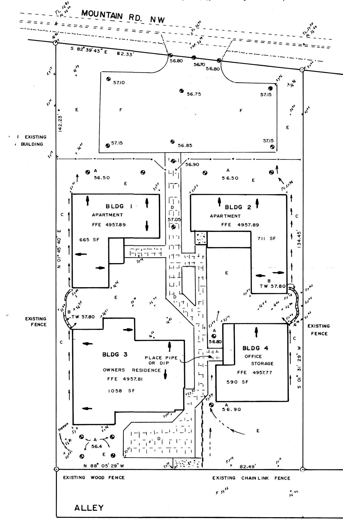
The purpose of this grading and drainage plan is to obtain approval for a occupancy of apartment dwellings on lot 408-A.
