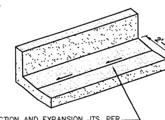
CONTRACTION AND EXPANSION JTS. PER -C.O.A. MEDIAN CURB DETAIL, SEAL WITH WATERTIGHT SEALANT.
