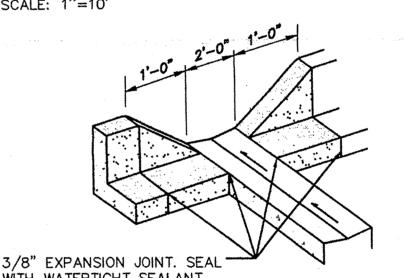
WITH WATERTIGHT SEALANT. REMOVE ALL EDGES WITH 3/8"
