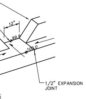
1. EDGES NOT SPECIFICALLY DIMENSIONED SHALL BE SHAPED WITH A 3/8" EDGING TOOL.
