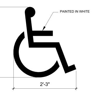
HC PAVEMENT MARKING SCALE: NTS
