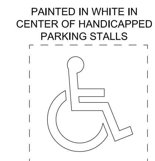
ACCESSIBLE PARKING SPACE MARKING DETAIL
