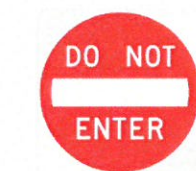
"DO NOT ENTER" SIGN (R5-1) DETAIL NTS
