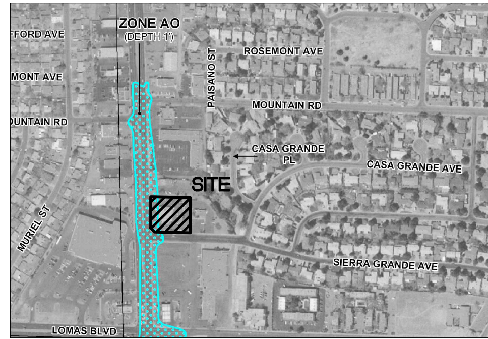
FIRM MAP 35001C0359G Per FIRM Map 35001C0359G, dated September 26, 2008, the site is located in the Zone AO (Depth 1) Floodplain. The proposed building is not located within the Zone AO designated area.
