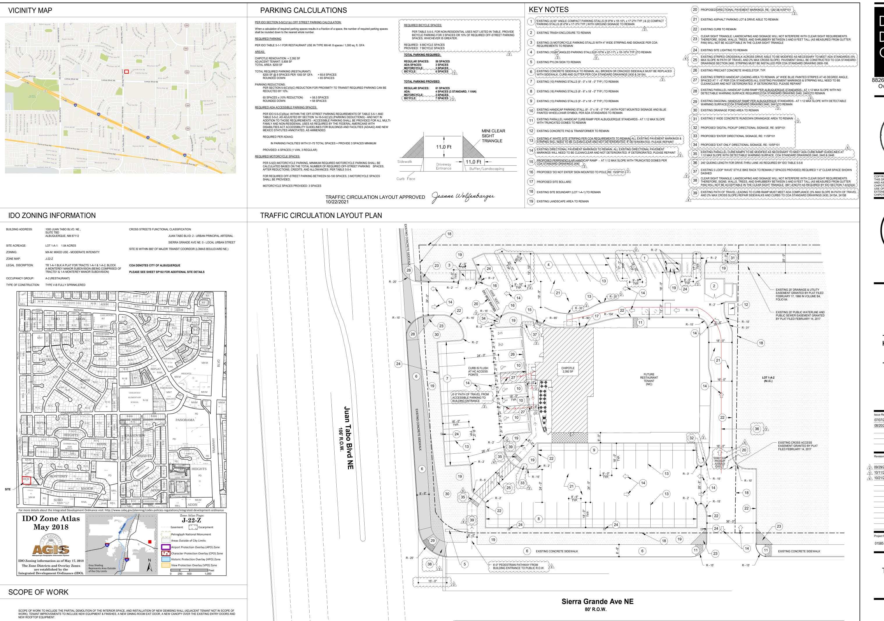
ALL SITE WORK INCLUDING PAVING, CURBING, PARKING, SIDEWALKS, LANDSCAPING, DUMPSTER ENCLOSURE, AND PARKING LOT LIGHTING ARE EXISTING AND ASSUMED COMPLIANT TO REMAIN. PROPOSED SITE MODIFICATIONS INCLUDE (2) 'DO NOT ENTER' POST MOUNTED SIGNS, (1) ADA RAMP AND NEW PAVEMENT
