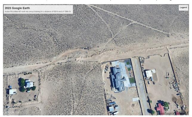
The 3/18/25 Google Earth image below shows an additional berm at the  $104^{th}$  St. trail crossing Avalon Rd. blocking flows that would otherwise flow into the new pond at  $102^{nd}$  St., constructed in 2024 as part of Paradise RV Park Phase 2.
