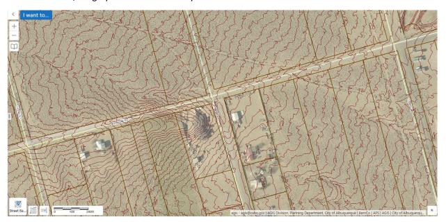
The 5/7/23 Google Earth image shows the Avalon roadway shifted 60 feet north at the arroyo location for a 500-foot stretch west of 106th St., and extensive berms were built to prevent the arroyo from spreading south.
