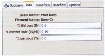
Figure 106. Initial and constant loss method editor.
