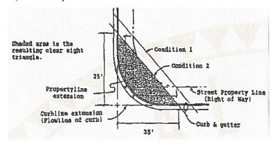
8. Please add the following note to the clear sight triangle: "Landscaping and signage will not interfere with clear sight requirements. Therefore, signs, walls, trees, and shrubbery between 3 and 8 feet tall (as measured from the gutter pan) will not be acceptable in this area."
