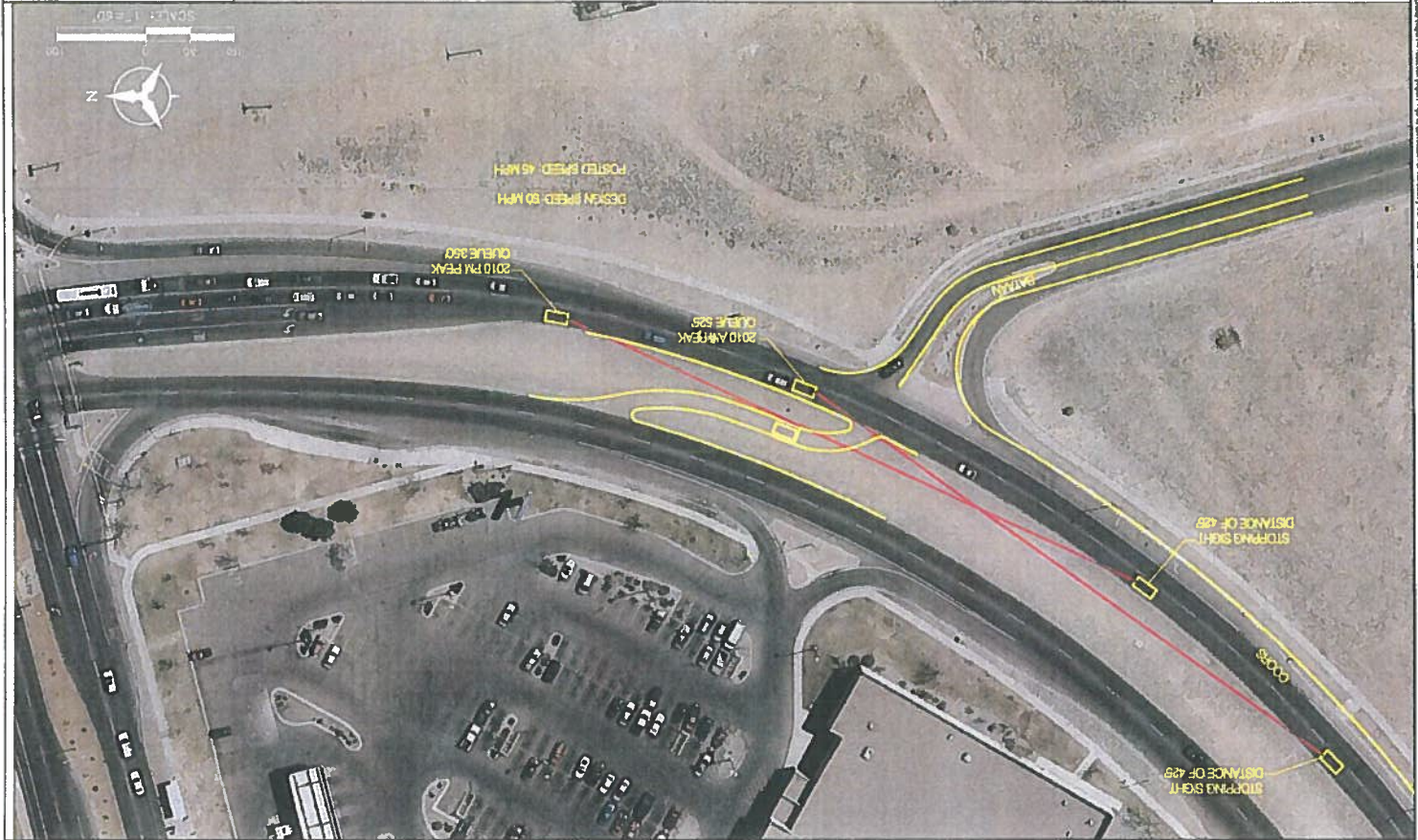
FIGURE 1 SIGHT DISTANCE REQUIRED 50 MPH DESIGN SPEED
