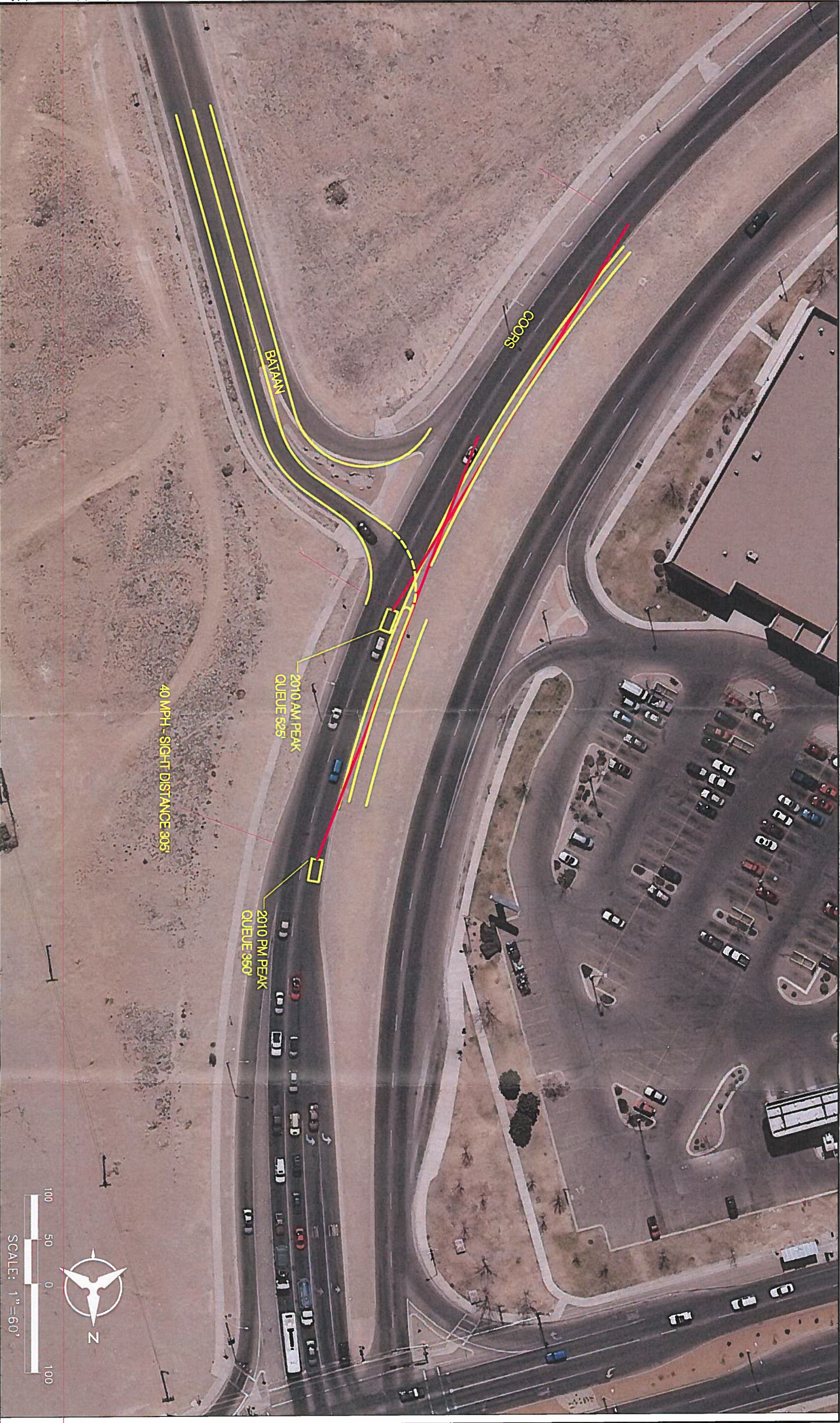
FIGURE 3 SIGHT DISTANCE REQUIRED 45 MPH DESIGN SPEED
