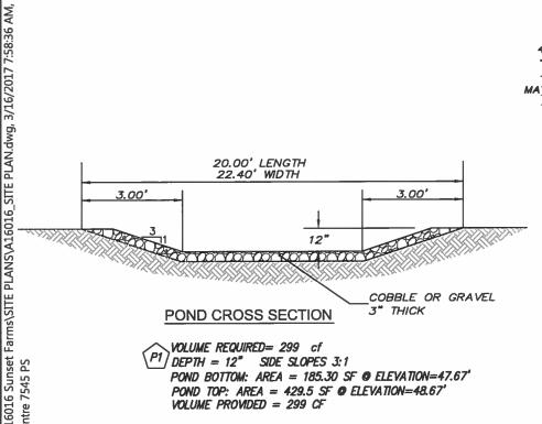
P1 VOLUME REQUIRED= 299 cf SIDE SLOPES 3:1 POND BOTTOM: AREA = 185.30 SF @ ELEVATION=47.67 POND TOP: AREA = 429.5 SF @ ELEVATION=48.67\*
