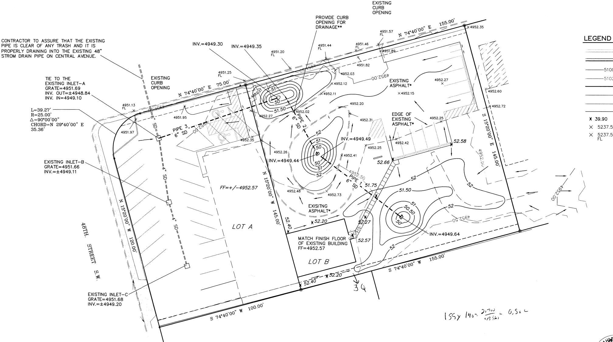
— EXISTING CONTOUR (MAJOR) —— EXISTING CONTOUR (MINOR) BOUNDARY LINE - EASEMENT LIMITS OF TOP OF EXISTING SLOPE - EXISTING FENCE X 39.90 PROPOSED GRADE × 5237.50 EXISTING GRADE × <u>5</u>237.50 EXISTING GRADE (FLOW LINE)
