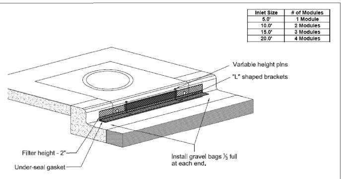
Definition - ERTEC Curb Inlet Guard
