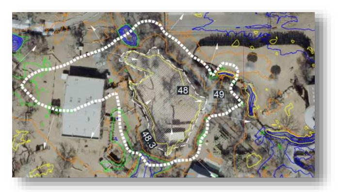
At a FF elevation of 4949.0, the proposed building will displace approximately 4800 cf. The result will be raise the maximum water surface elevation (100-year 10-day storm event) approximately 0.2' to 4948.5.
