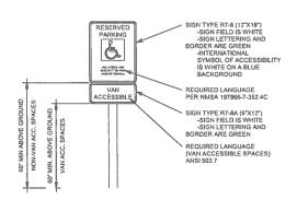
ALL SIGNS SHALL COMPLY WITH U.S. DEPARTMENT OF TRANSPORTATION, FEDERAL HIGHWAY ADMINISTRATIONS "MANUAL OF UNIFORM TRAFFIC CONTROL DEVICES", LOCAL CODES AND AS SPECIFIED. MOUNT SIGNS TO POST IN ACCORDANCE WITH MANUFACTURER'S INSTRUCTIONS.
