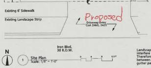
Landscaping, fencing, and signage will not interfere with dear site triangle requirments. Therefore, signs, walls, trees, and shrubbery between 3 and 8 feet tall (as measured from gutter pan) will not be acceptable in this area
