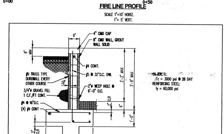
. RETAINING WALL SHALL NOT BE BACK-FILLED UNTIL AT LEAST 7 DAYS AFTER GROUTING THE WALL. 2. LAP SPLICE ON REINFORCING BARS IS NOT ALLOWED
