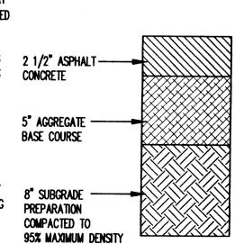
8" SUBGRADE PREPARATION COMPACTED TO 95% MAXIMUM DENSITY LIGHT DUTY PAVEMENT SECTION
