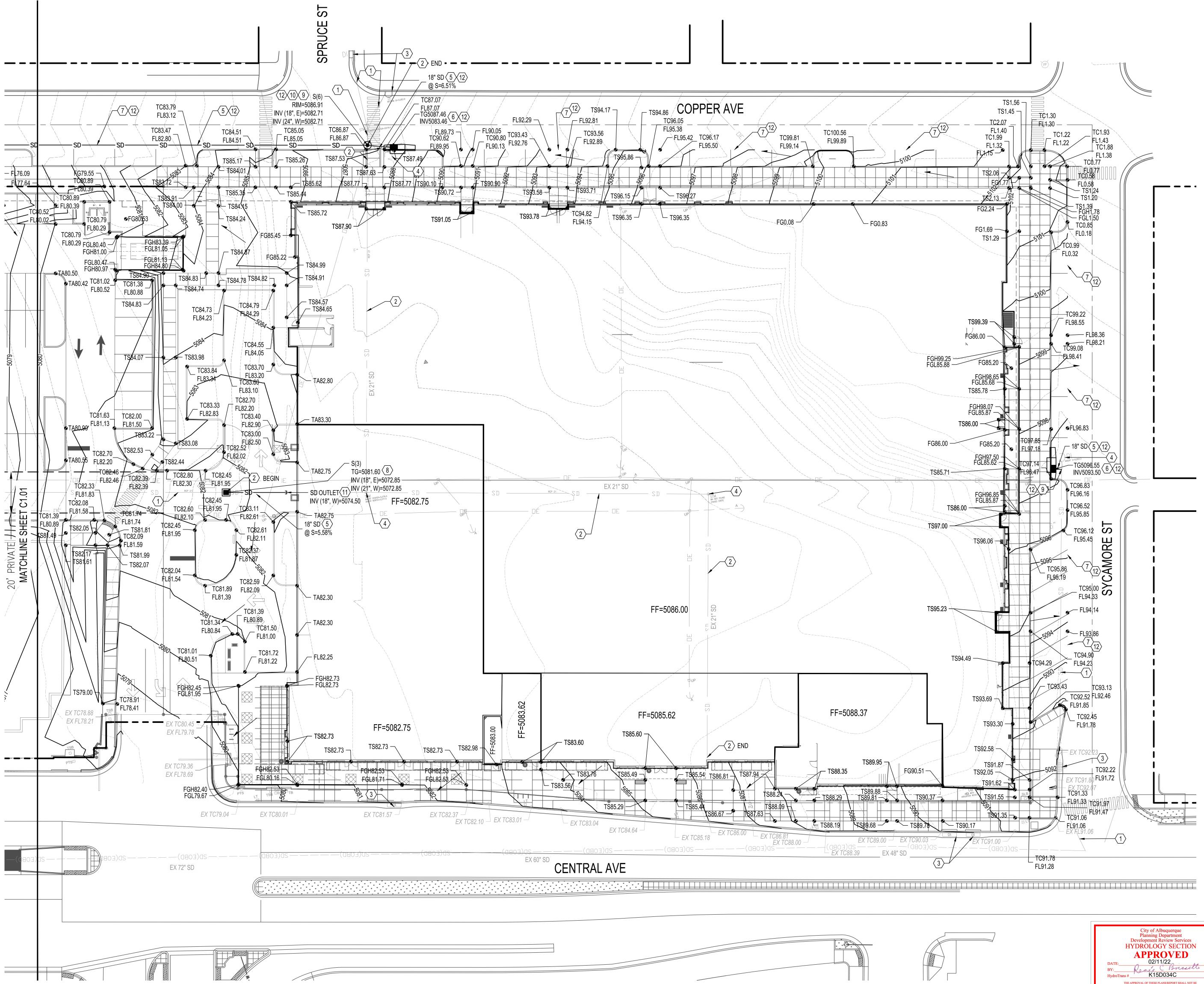
HDPE PIPE AND FITTINGS SHALL BE INSTALLED AN DBACKFILLED PER MANUFACTURER SPECIFICATIONS. CONNECTIONS TO CONCRETE MANHOLES AND CONCRETE DROP INLETS SHALL USE WATER STOP GASKETS AND SHALL BE INSTALLED PER MANUFACTURER'S SPECIFICATIONS.
