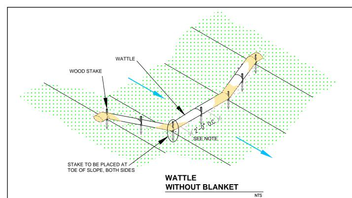
2' FOR DRAWING ONLY. 8' MAX SPACING BETWEEN STAKES
