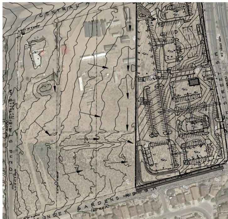
Offsite Drainage Path (Bernalillo County 2-foot Contours)
