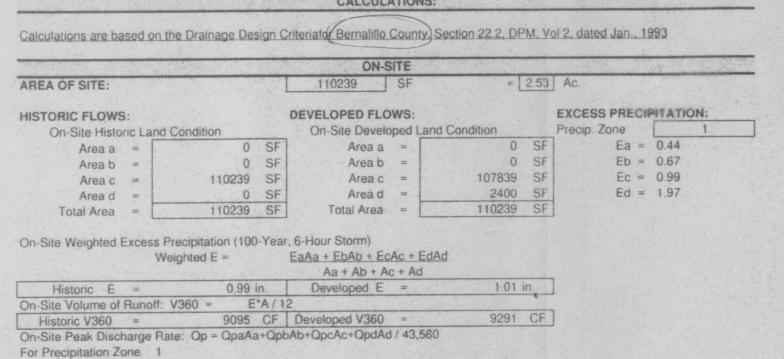
Excess Flows to be ponded on North side of proposed gravel road = DISPLACED VOLUME CALCULATIONS Based on the F.I.R.M. Map #33, the floodzone for this property is designated as AO which is an area of 100-year shallow flooding where
