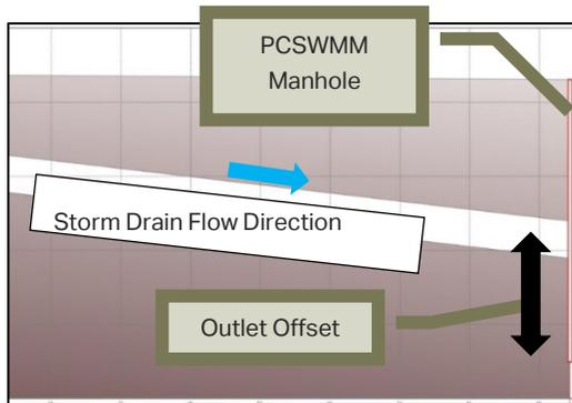
Figure 12: Storm Drain with Outlet Offset Example
