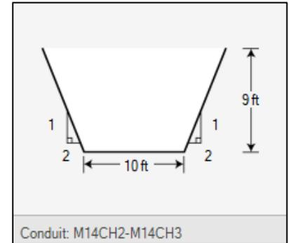
Figure 15: Channel Schematic Example
