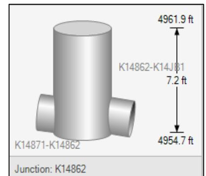
Figure 16: Manhole Schematic Example
