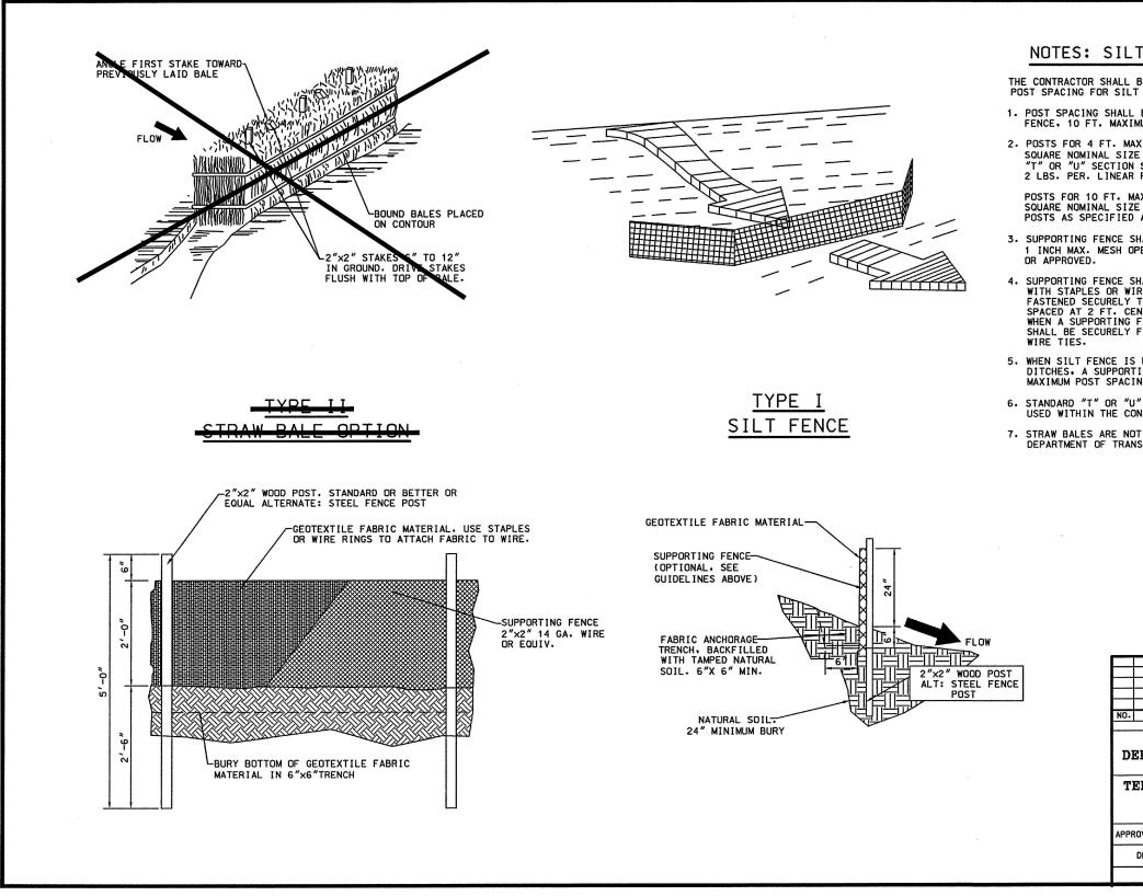
TEMPORARY EROSION AND SEDIMENT CONTROL MEASURES PLAN DETAILS SCALE: 1" = 20'
