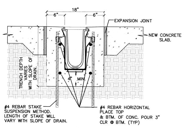
SET TRENCH DRAIN IN CHANNEL SURROUNDED BY 6" OF CONCRETE OR THICKNESS OF THE CONCRETE SLAB WITH A MINIMUM OF 3,500 P.S.I. AVOID FULL LOAD TRAFFIC FOR 28 DAYS OR UNTIL CONCRETE HAS COMPLETELY HARDENED.
