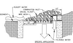
THIS METHOD OF INLET PROTECTION IS APPLICABLE AT COMBINATION INLETS WHERE PONDING IN FRONT OF THE STRUCTURE IS NOT LIKELY TO CAUSE INCONVENIENCE OR DAMAGE TO ADJACENT STRUCTURES AND UNPROTECTED AREAS.
