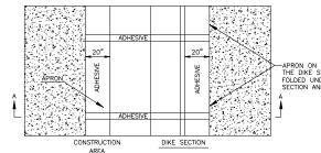
ADHESIVE SHALL BE PLACED WHERE THE UNITS OVERLAP AND A 20" STRIP ALONG BOTH EDGES.
