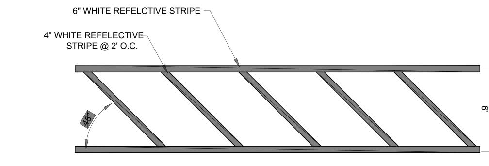
1. CROSSWALK ALONG AN ACCESSIBLE ROUTE SHALL MAINTAIN A SLOPE OF 2% MAX. IN ALL
