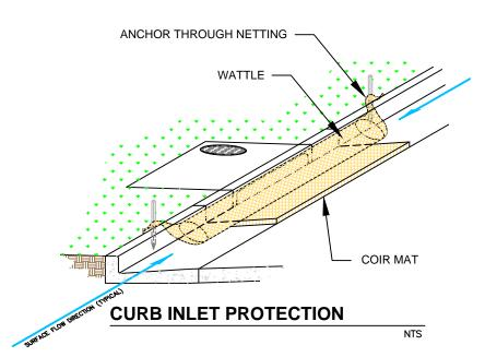
THE MAT SHOULD EXTEND A MINIMUM OF 1" PAST ALL EDGES OF THE INLET. PLACE MAT AGAINST THE CURB INLET.
