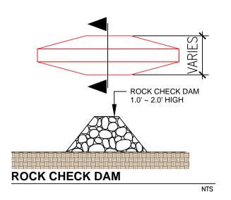
PLACE CHECK DAMS AT REGULARLY SPACED INTERVALS ALONG SWALE OR DRAINAGE DITCH.
