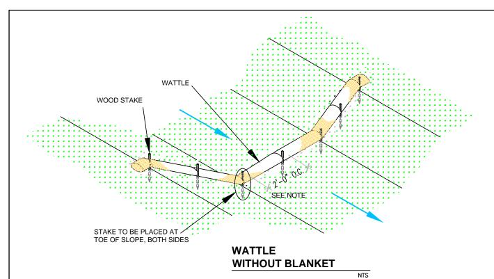
2' FOR DRAWING ONLY. 8' MAX SPACING BETWEEN STAKES
