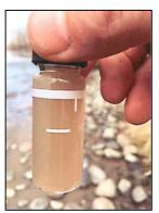
Figure 5. Turbidity sample collected in a cuvette.
