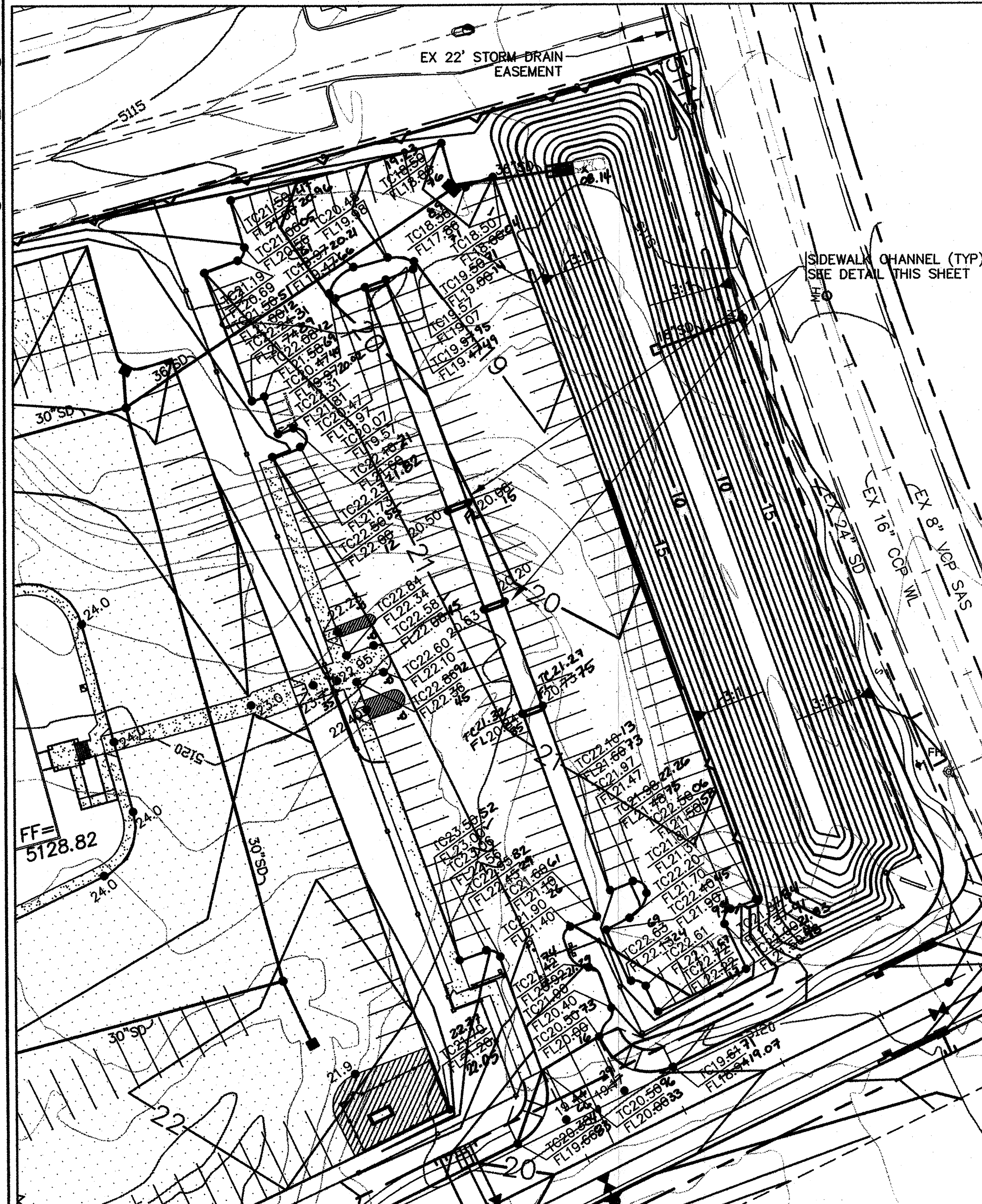
STANDARD VEHICLE PARKING LOT - ENLARGED GRADING DETAIL SCALE: 1" = 40'
