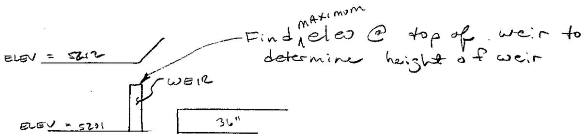
MAX Q thru 36" RCP w/ Water Surface at elev 5212 (spillway)
