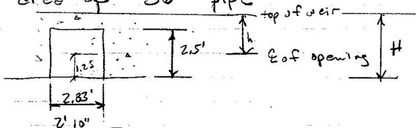
orifice equation  $Q = C_d \sqrt{2gh}$
