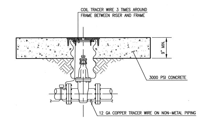
(A1) TYPICAL WATER VALVE BOX SECTION
