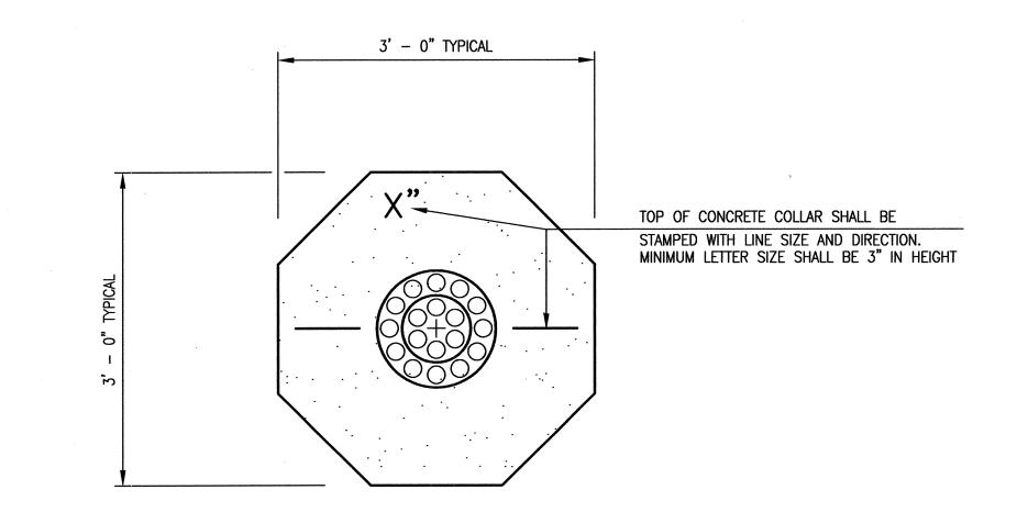
(C1) TYPICAL WATER VALVE BOX COLLAR DETAIL
