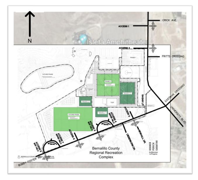
The anticipated implementation year for this project is 2026 and the horizon year is 2036. According to the Institute of Traffic Engineers' (ITE) trip generation rates, the project is anticipated to generate 102 new entering trips and 62 new exiting trips during the weekday AM Peak Hour
