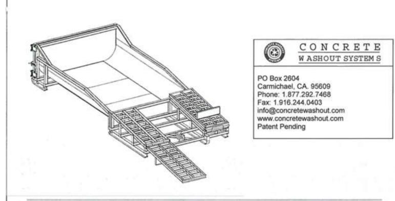
A portable, self-contained and watertight container affixed with ramps that controls, captures and contains caustic concrete wastewater and washout material.
