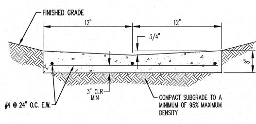
NOTE: IN DRIVE SURFACES VALLEY GUTTER SHALL BE POURED ON 4" ABC OVER 12" SUBGRADE PREP.
